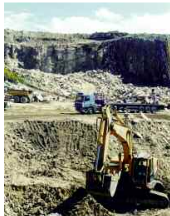
The quarry at Clashach, with sloping dune bedding visible on the quarry face.
